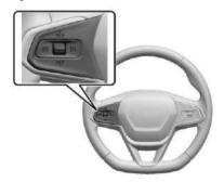
\*\*Press to turn cruise control on and off. The white cruise control indicator light comes on in the instrument cluster when cruise control is turned on.
