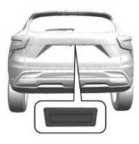
To open the liftgate, press the touch pad under the liftgate handle and lift up.
