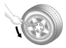
Turn the wheel wrench counterclockwise to loosen the wheel nuts. Do not remove them yet.
