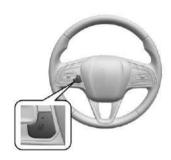
: If equipped with a heated steering wheel, press to turn on or off. A light near the button displays when the feature is turned on.
