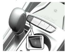
The automatic engine stop/start feature can be disabled and enabled by pressing  $\widehat{\mathbf{o}}_{\text{FF}}^{(A)}$ . Auto Stop is enabled each time you start the vehicle.
