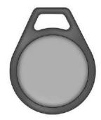
Interference from radio-frequency identification (RFID) tags may prevent the key from starting the vehicle. Keep RFID tags away from the key when starting the vehicle. The key that is part of the Remote Keyless Entry (RKE) transmitter can be used for the ignition and all locks.
