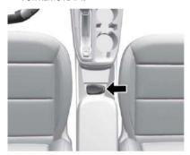
4. Place the new transmitter in transmitter pocket.
