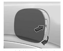
To open the fuel door, push and release the rearward center edge of the door.
