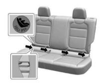
The ISOFIX anchors are located near the crease between the seatback and the seat cushion and identified with the symbol .
