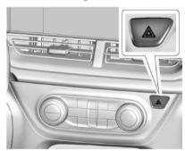
in Press to make the front and rear turn signal lamps flash on and off. This warns others that you are having trouble. Press again to turn the flashers off.
