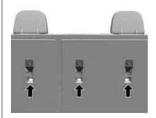
Top tether anchors are located on the back of the second row seatbacks and are always aligned with rear seats and identified with symbol .
