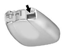
Separate the two halves of the transmitter using a flat tool inserted into the area near the key slot.
