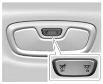
If equipped, the rear dome lamp controls are in the headliner above the rear seats.
