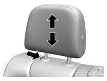
To lower the head restraint, press the button on the top of the seatback and push the head restraint down. Try to move the head restraint after the button is released to make sure it is locked in place.
