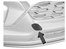
Carefully open the cover on the fascia by using the small notch that conceals the tow eye socket.
