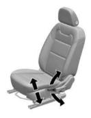
If available, move the lever up or down to manually raise or lower the seat.
