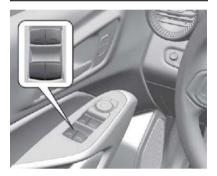
The power windows work when the vehicle is on or when Retained Accessory Power (RAP) is active. See Retained Accessory Power (RAP)
