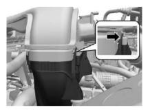
2. Disassemble the duct.
