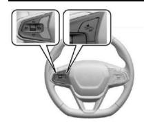
ress to turn the system on or off. The indicator turns white on the instrument cluster when ACC is turned on.
