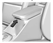
There is storage under the armrest in the center console. Press the button and lift to open.
