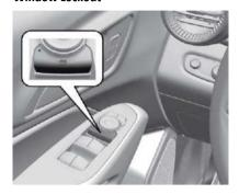
This feature stops the rear passenger window switches from working.
