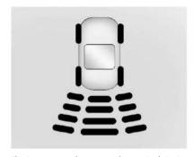
The instrument cluster may have a Park Assist display with bars that show "distance to object" and object location information for the Park Assist system. As the object gets closer, more bars light up and the bars change color from yellow to amber to red.
