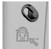
If equipped, the safety lock is on the inside edge of the rear doors. To use the safety lock:
