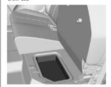
Crew cab models have storage compartments under the bottom of the rear seats cushion.
