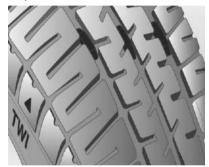
Tires must also be replaced when their tread depth has worn down near to 1.6 mm. The image shows where the tread depth can be found.
