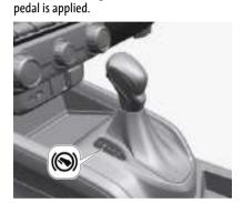
Without brake pedal applied, the control indicator (S) illuminates.
