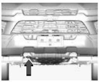
The towing eye is located at the front of the vehicle under the bumper.
