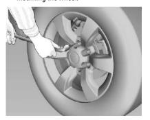
Turn the wheel wrench counterclockwise to loosen all the wheel nuts. Do not remove the wheel nuts uet.
