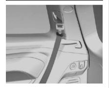
Guide the seat belts through the belt holders to ensure that the third row seats do not get stuck while the seats are raised.
