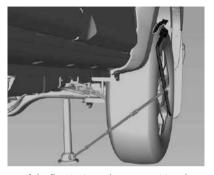
If the flat tire is on the rear, position the jack under the rear axle and get as close as possible to the shock absorber.
