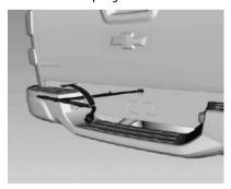
Turn the wheel wrench counterclockwise to lower the spare tire to the ground. Continue to turn the wheel wrench until the spare tire can be pulled out from under the vehicle.
