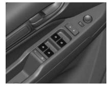
Operate the switch for its respective window by pushing to open or pulling to close. The switch for the driver's window has a light which signals through illumination the operation readiness.
