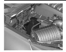
If the cooling system is cold, the coolant level should be about 1cm above the filling line mark. Top up if the level is low.
