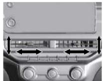
Push the adjuster knob up to right and left to close the vent or to adjust the volume of air.
