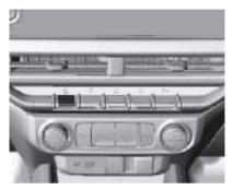
At speeds below 30 km/h (19 mph), press button . The green control indicator will turn on in the instrument panel. The green control indicator will flash in the instrument panel when the HDC is in operation. HDC will neither activate nor operate at speeds above 30 km/h (19 mph), even if the button is pressed.
