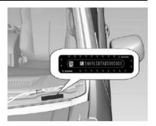
The Vehicle Identification Number is embossed on the instrument panel visible through the windscreen.
