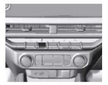
For very high-performance driving, ESC can be deactivated by pressing and holding ab button and a message will appear on the Driver Information Center (DIC).
