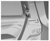
Guide the seat belts through the belt holders to ensure that the third row seats do not get stuck during stowing of the seats.
