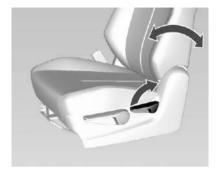
Pull the lever, adjust the inclination and release the lever. The seat should lock into place. Try to move the seat back and forth to ensure that the seat is locked in place.
