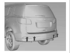
The parking assist makes parking easier by measuring the distance between the vehicle and the obstacles and giving acoustic signals. It is the driver, however, who bears full responsibility for the parking maneuver.
