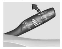
The rear window wiper only operate with the ignition on or accessory mode.
