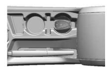
Place the non-remote key or the transmitter in the center console or in the armrest. The correct positions are shown in the figures.
