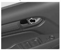
Push the locking button of the respective doors inwards. These doors will be locked.
