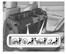
The seat position instruction is displayed on a label on the back of the seat.
