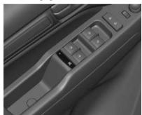
Press switch at to deactivate the power windows of the rear doors. The other power windows can be operated by switches on the driver's door.
