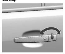
Manually unlock the driver's door by turning the key clockwise. Switch on the ignition to deactivate the anti-theft alarm system and press the central locking button to unlock all doors and liftgate.
