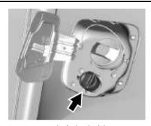
Do not remove the fuel and AdBlue caps at the same time. Fill diesel fuel and AdBlue independently.
