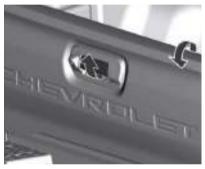
To open, pull the center handle and lower the tailgate. To close, raise the tailgate and press the upper ends until hearing a locking noise.
