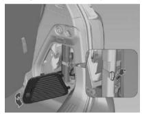
To release the tools, the strap has to be unhooked and the jack has to be retracted.
