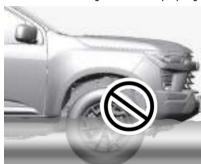
Drive at low speed through any flooded area and make sure the water limit does not exceed the wheel center of height.
