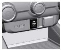
If equipped the rear air conditioning system is operated with the **REAR A/C** button.
