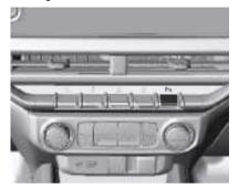
The PM button of the instrument panel is used to turn on or off the Front and Rear Parking Assist. The indicator LED next to the button comes on when the features are on and turns off when the features have been disabled. Turn off parking assist when towing a trailer.
