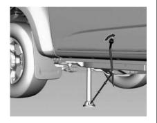
If the flat tire is on the front of the vehicle, position the jack to the rear of the front tire in the pocket off of the frame.
