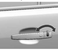
To lock the driver's door, turn the key counterclockwise.
