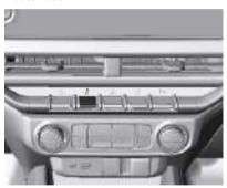
Traction Control can be switched off when spinning of the traction wheel is required by pressing & button and a message will appear on the Driver Information Center (DIC).
