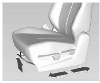
Pull the handle, slide the seat, release the handle. Try to move the seat back and forth to ensure that the seat is locked in place.
