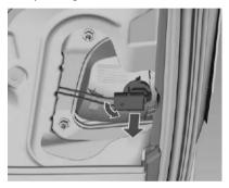
Rotate the relevant bulb holder counterclockwise and remove it.
