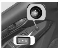
Move the selector switch to the L (left) or R (right) to choose the driver or passenger mirror. Move the mirror to the desired direction by pressing the four-way switch.
