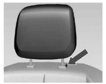
Pull the head restraint upward.
