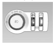
To adapt headlight range to the vehicle load to prevent dazzling, turn the knob to the required position.
