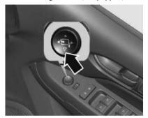
Press the selector switch (L / R switch) to the central position, then press the four-way switch to power fold the mirrors. Press again to unfold.
