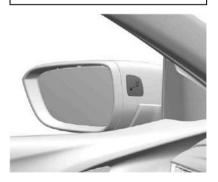
When the vehicle speed is higher than 10 km/h, the side blind spot alert system will be activated. When the vehicle speed is more than 140 km/h, the system will be turned off, and the indicator lamp of the left and right exterior mirrors will dim; at this time, if the vehicle speed is reduced, the indicator lamp of the mirror will be extinguished. If a vehicle is detected in the blind spot at this time, the indicator lamp of the corresponding rearview mirror will illuminate.
