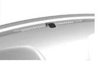
There is a light sensor on top of the instrument panel. Do not cover the sensor.
