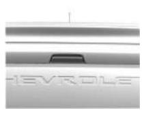
To open the tailgate, the vehicle must be off or stopped, with the shift lever in P (Park), if equipped.
