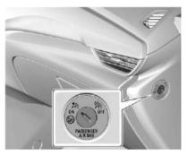
Front passenger airbag system can be deactivated via a lock on the side of the instrument panel, visible when the front passenger door is open.
