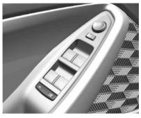
Press the switch at to deactivate rear door power windows switch. To activate, press again.
