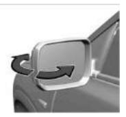
For pedestrian safety, the exterior mirrors will swing out of their normal mounting position if they are struck with sufficient force. Reposition the mirror by applying slight pressure to the mirror housing. This feature is also useful to reduce the total width of the vehicle to prevent damages when the vehicle is parked. Push the mirror back into the functional position before driving.
