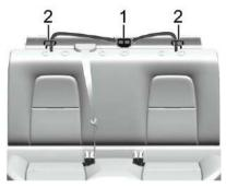
The top tether is routed through loops (2) to the top tether anchor (1). Be sure to read the following instructions to properly install a child restraint using these loops and anchor.
