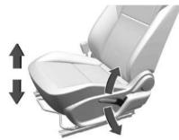
If equipped, move the lever up or down to raise or lower the seat.
