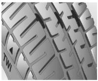
Tyres must also be replaced when their tread depth has worn down near to the TWI. The image shows where the tread depth can be found.
