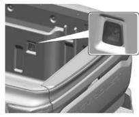
If equipped, the exterior cargo lamp is located on the inner side panel and has the function of illuminating the cargo area.
