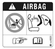
NEVER use a rearward-facing child restraint on a seat protected by an ACTIVE AIRBAG in front of it; FATAL or SERIOUS INJURY to the CHILD can occur.
