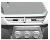
Use the fins on the air vents to change the direction of the airflow.
