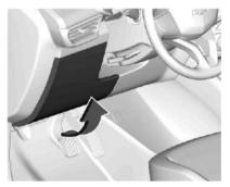
The instrument panel fuse block is located on the underside of the driver's side instrument panel.
