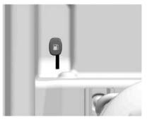
Pull up the small fuel door handle on the left side of the driver seat to open the small fuel door.
