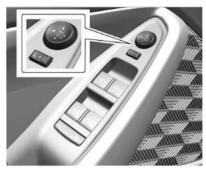
If equipped, the control for the power mirrors are located on the door trim beside the driver.
