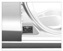
The vehicle Identification Plate is located on the right front door pillar.
