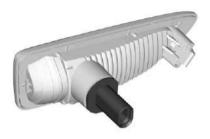
Rotate the bulb holder counterclockwise to disengage it.
