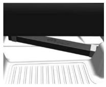
The Warning Triangle is stored under the front passengers seat.
