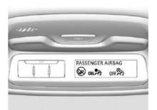
As long as the control indicator  $\overset{\circ}{\sim}$  is illuminated, the airbag systems for the front passenger seat will inflate in the event of a collision.
