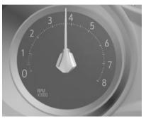
The tachometer displays the engine speed in revolutions per minute (rpm).
