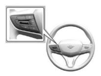
The speed limiter button is on the steering wheel.
