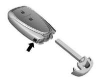
Press the button on the side of the detachable key and pull the mechanical key out. Never pull the key out without pressing the button.
