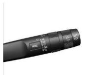
Press MENU to switch between the main menus or to return from a submenu to the next higher menu level.
