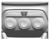
$\triangle$ : Press  $\triangle$  to make the front, rear and side turn signal lamps flash on and off. Press again to turn the flashers off.
