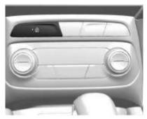
**•** : Press to lock the doors. The indicator light will come on when the door is locked. To unlock the door, press the switch again.
