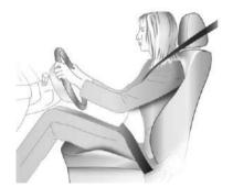
Sit as far back against the backrest as possible. Adjust the distance between the seat and the pedals so that your legs are slightly angled when pressing the pedals.
