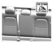
Top tether anchor is located behind the rear seat center head restraint and is identified with the symbol 🏝 on the rear panel.
