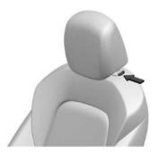
Pull the head restraint up to raise it. Try to move the head restraint to make sure that it is locked in place.
