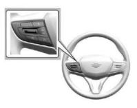
S: Press to turn the cruise control system on and off. A white indicator comes on in the instrument cluster when cruise is turned on.
