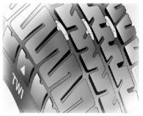
The legally permissible minimum tread depth (1.6 mm) has been reached when the tread has worn down as far as one of the tread wear indicators (TWI). Their position is indicated by markings on the sidewall. Tyres age, even if they are not used. We recommend tyre replacement every 6 years.
