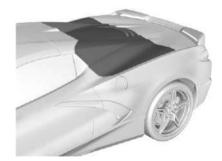
Hold the tonneau cover is completely closed. A chime will sound, a DIC message will display, and the turn signals will flash once.
