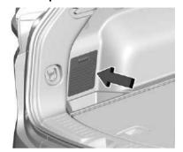
The rear compartment fuse block is behind a trim cover on the driver side of the rear storage compartment. Remove the trim cover to access the fuse block or visit your dealer.
