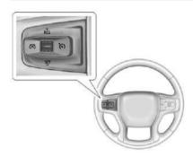
ress to turn cruise control on or off. A white indicator light is displayed in the instrument cluster when cruise control is turned on.
