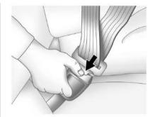
To unlatch the belt, push the release pushbutton on the buckle. The belt should return to its stowed position.
