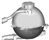
Check to see if coolant is visible in the coolant surge tank. If the coolant inside the coolant surge tank is boiling, do not do anything else until it cools down. See Engine Overheating
