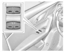
The power windows work when the vehicle is on, in accessory mode, or when Retained Accessory Power (RAP) is active. See *Retained Accessory Power (RAP)* ⇔ 188.
