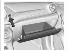
To open, press the button. Close the glove box manually.
