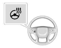
: If equipped, press to turn the heated steering wheel on or off. A light next to the button displays when the feature is turned on.
