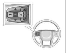
(c): Press to turn the system on or off. The indicator turns white on the instrument cluster when ACC is turned on.
