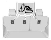
Top tether anchors are located on the back of the second row seatbacks and are always aligned with rear seats and identified with the symbol ...
