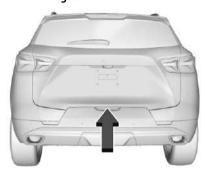
To open the liftgate, press the touch pad in the liftgate handle and lift up. Unlocking all doors will also unlock the liftgate.
