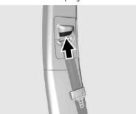
Press and hold the release button while raising or lowering the height adjuster to the desired position.
