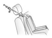
If the position you are using has an adjustable head restraint and you are using a single tether, raise the head restraint and route the tether under the head restraint and in between the head restraint posts.
