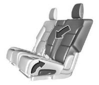
Pull the handle on the side of the seat cushion to unlock it. Fold the seatback forward.
