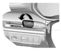
To switch on or off the headlamp, tail lamp and parking lamp, turn the end of the combination switch control lever.
