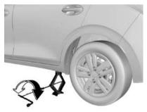
Rotate the jack rocker clockwise to allow the jack to rise slowly and ensure that the jack head is firmly pushed into the lifting position.
