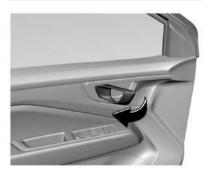
To open doors from inside or outside, unlock the doors first, and pull the external or internal door handles.
