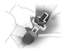
Pull the seat belt out of the retractor, guide it around the body without twisting, and insert the locking tab into the buckle to fix it. When driving, pull the shoulder belt forcibly to adjust the tightness of hip belt.
