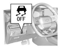
Press the ESC OFF switch, and the ESC OFF lamp on the instrument cluster illuminates and some ESC functions are disabled. Press the ESC switch again, the ESC function is enabled again and the ESC OFF lamp on the instrument cluster goes out.
