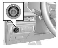
The power outside rearview mirror adjustment switch is on the left side of the instrument panel.
