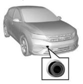
The front towing hook has a hole cover on the right side of the bumper, and the fixing hole for installing the towing hook can be seen by opening the hole cover. Place the towing hook in the tool bag of the luggage compartment. Take out the towing hook and install it into the fixing hole. Rotate the towing hook clockwise to tighten it completely and insert a socket wrench into the hook hole to assist tightening. Be sure that the towing hook is installed firmly before towing the vehicle.
