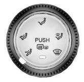
Adjust the air distribution knob to the desired mode so that the air flows in the desired direction.
