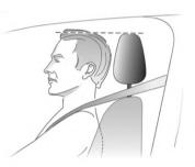
The middle position of the headrest should be on the same horizontal line as the occupant's eyes. For tall persons, if the above point cannot be met, the headrest should be adjusted to the highest position; for short persons, the headrest should be adjusted to the lowest position.
