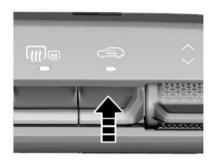
When the ignition is turned on, press this button to switch between the air inner and outer circulation modes. When using the inner loop mode, the indicator above the inner loop button illuminates. The outer or inner loop status is displayed on the multimedia accordingly.
