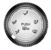
To turn on the defroster, first turn on the ignition and then press the rear windshield defroster button. The indicator under the button illuminates. Press again to turn off the defroster and the indicator under the button turns off.
