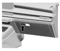
Pull the handle outward to open it. To close, push and fasten the glove box door inward.
