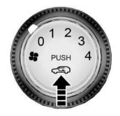
Press this button during when on a dusty road, or when you want to prevent the exhaust or outside smoke entering inside, or when you want to quickly decrease temperature in the passenger area.
