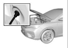
3. Separate the engine hood prop rod from the fixing clamp. Lift the prop rod up and firmly insert the free end into the slot on the engine hood.
