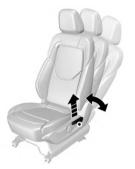
Pull up the lever and adjust the tilt angle of the backrest to a proper position, and then release the lever. Do not lean on the seat backrest while adjusting. After adjusting the backrest, lean back on it to ensure that the it is locked in place.
