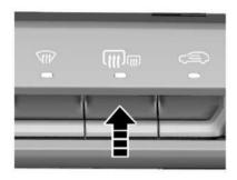
To turn on the defroster, first turn on the ignition and then press the rear windshield defroster button. The indicator above the button illuminates, and the corresponding working status will be displayed on the multimedia
