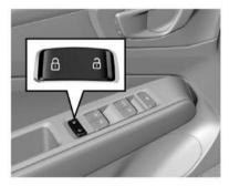
To lock the doors from inside the vehicle, press to n the door handle. To unlock the doors from inside the vehicle, press i on the door handle.
