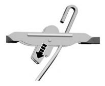
As shown, adjust the wiper blade to an angle perpendicular to the wiper arm, and then press the blade in the direction of the arrow to separate the blade from the wiper arm.
