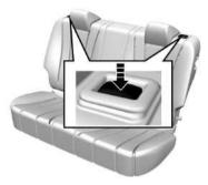
Flip the cushion first, then pull the backrest strap to unlock the backrest, and then fold the backrest forward until it is flat. Both backrests can be folded and laid flat. Operate in the reverse order when restoring. Try to shake the backrest and cushion to ensure that they are locked.
