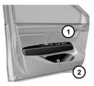
The door storage groove (2) and armrest (1) are located on inner side of the door panel.
