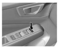
The electric window lock button can be pressed to lock the rear windows and the front passenger window switch. When the button is pressed, the rear windows and front passenger side window can only be controlled by the window control panel on the driver side. Press again to unlock.
