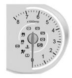
It displays the engine crankshaft revolutions per minute.
