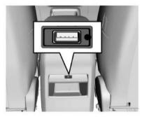
If the vehicle is equipped with rear accessory USB power outlet (5 V), it is located at the rear of the console. It can be used for charging mobile phones. The power outlet is unavailable if the ignition is turned off.
