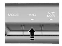
To turn on, press the A/C button, the indicator above the button illuminates, and the corresponding working status will be displayed on the multimedia. The air conditioner performs the cooling function.
