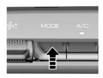
When the blower is on, press the mode selection button, the blowing mode can be switched in the order of "faceblowing — face/foot-blowing—foot-blowing —foot-blowing/defrosting—face-blowing".
