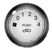
Turn the fan speed control knob to control the system air flow.
