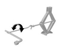
4. Connect the wheel nut wrench and jack rocker to the jack as shown.
