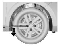
1. Use a socket spanner to unscrew the wheel nut by one turn.
