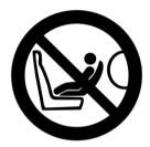
Do not use a backward-facing child restraint system on a seat (front seat) protected by a frontal airbag (in the activated state). Otherwise, severe injuries or even death may be caused to the child when the airbag is deployed.
