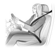
The seat belt is designed only for one passenger. It is not applicable to a passenger under 12 years old or under 150 cm high. Check all parts of the seat belt system for damage and abnormal function regularly. Replace the damaged parts and components. To replace or service a seat belt, see your dealer.
