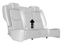
Pull the back of the seat cushion slightly to unlock and lift the seat cushion.
