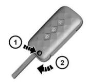
Press the release button, and the mechanical key will automatically extend open. Fold the mechanical key after use.
