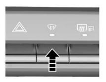
Press the front defrost button to turn on the front windshield defrost mode. The indicator above the button illuminates, and the corresponding working status will be displayed on the multimedia.
