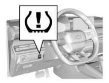
For an indirect TPMS vehicle, a tire pressure reset learning must be carried out after the tire pressure is adjusted or a tire is replaced.
