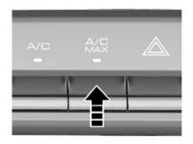
When the engine starts, press the A/C Max button to turn on the extreme cold mode.
