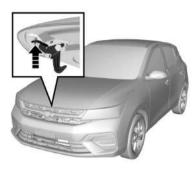
Reach your hand to the lower side of the engine hood front edge, as shown above, and lift the engine hood release handle up. Lift up and fully open the engine hood.
