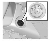
When the ignition is turned at the right side of the steering column, the operating positions are as follows:
