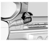
When the headlamp is in low beam or the front fog lamp is turned on, turn the rear fog lamp
