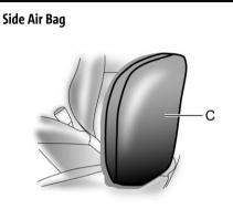
As shown in Figure C above, the front seat side airbag is installed on the backrest side near to the door.
