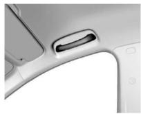
The auxiliary handrail is convenient for passengers to get in and out of the vehicle. The passengers can also grab the handrail to help maintain the sitting position when the vehicle speed is fast.
