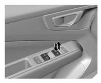
To raise the window, pull upward the switch. To lower the window, press down the switch. When the window reaches the desired position, release the switch.
