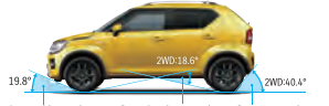
Approaching angle (excluding air dam) 19.8° Ramp breakover angle ZWD:18.6° Departure angle ZWD:40.4°
