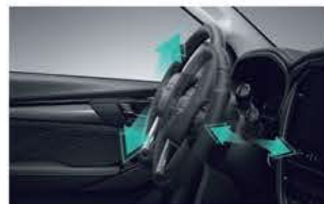
Multi-functional Steering Wheel with Tilt and Telescopic function are ergonomically designed for convenience of driving and intuitive features control.
